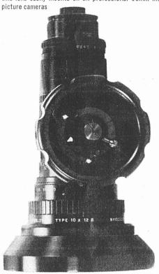
aperture: f:2.2/fixed image plane at all focal lengths /zoom range: 12mm to 120mm/weight: one pound, 14 ounces/length: 53/4 inches. Package prices including custom made deep bore sunshade-filter holder. two close-up lenses-+1 and +2 and one #85 color filter ...
